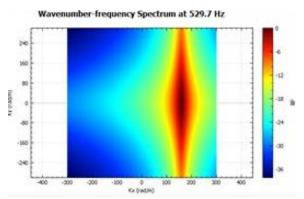
Image: New, robust, easy-to-use tools in the <u>VA One AVA module</u> allow data to be processed and convert the pressures to a wavenumber-frequency spectrum, which can be applied as a load to the vibroacoustic model to predict interior wind noise.
