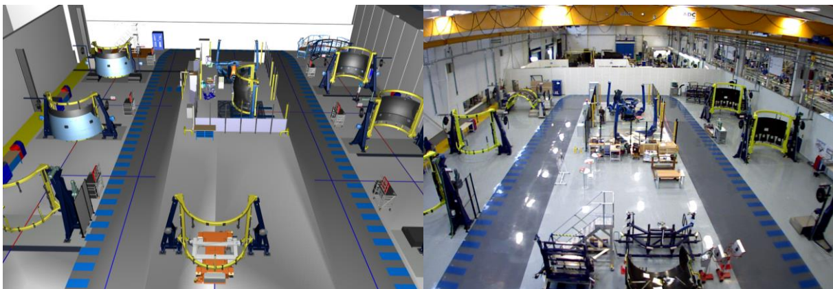
Image: Transcowl A330neo assembly line in Virtual Reality (left) and in reality (right).
